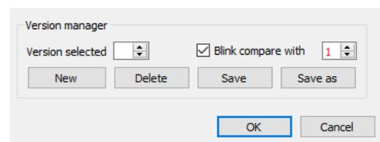
Once the user is satisfied with the selected version, pressing the "OK" button triggers PSS to save this image version along with the input image (as a 16bit .png, .tiff or .fits image). The file name is the one of the input image, extended by the suffix "\_gpp.png / .tiff / .fits". The parameters of all postprocessing versions and the number of the selected version are saved in the configuration file.
