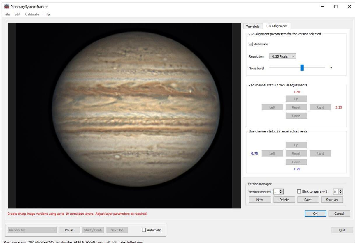
The red and blue figures in the channel status panels show the shifts applied to the red and blue channel in pixels.
