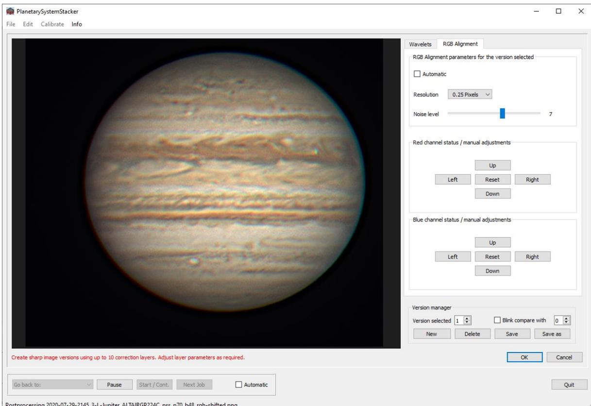
If, for example, the object was low in the sky during capturing, the three video color channels are misaligned due to differential atmospheric dispersion. As a result, color fringes appear at sharp edges such as planetary rims or lunar crater walls. PSS offers to shift the red and blue channels, relative to the green one, as part of the postprocessing pipeline.
